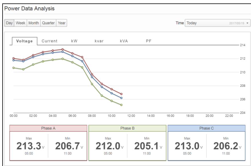
Figure 7-11 Historical Power Data - Power Data Analysis for Power Meter
